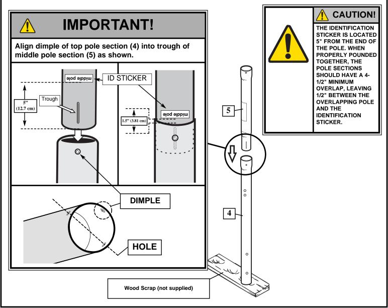
Bounce top and middle pole assembly (4 and 5) onto bottom pole section (6) using a wood scrap as shown. Bounce until the top and middle pole assembly no longer moves toward the pole identification mark on the bottom pole.
